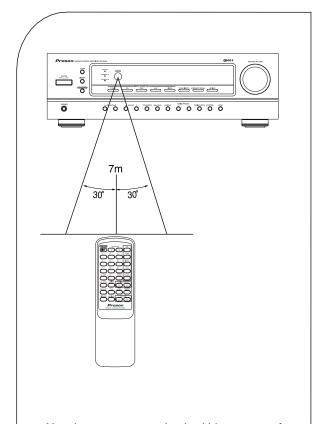
Use the remote control unit within a range of about 7 meters (23 feet) and angles of up to 30 degrees aiming at the remote sensor.
